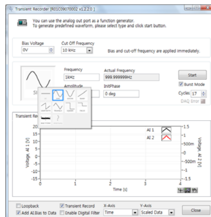
Transient recorder (Waveform generator) DC/Sine/Cosine/Ramp/Sawtooth/Square/Triangular/Pulse/ Multi-tone/ Arbitrary
